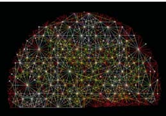
6. Generating an intriguing network of acrylic tubes for a proposed installation by combining a spatial tiling with evolutionary structural optimization (ESO). Colours indicate the iterations of the structural erosion process.
